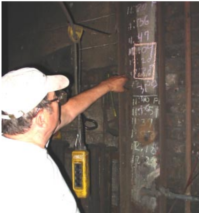
Photo 6. Bud Doebler pointing to record of pours during previous heat chalked onto wall near the cupola.
