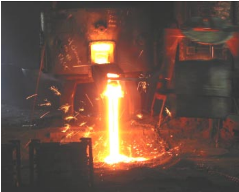
Photo 18. Excess iron being poured from the cupola into a pit in the foundry floor.
