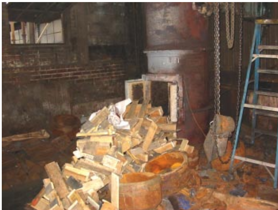
Photo 5. Newspaper, wood, coke, and iron to be charged through the charging doors in background. At the upper right can be seen part of an afterburner that combusts any carbon monoxide in the stack gases.
