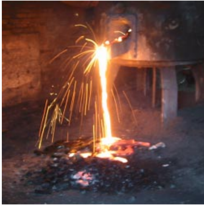
Photo 13. Slag flowing from the cupola's slag hole onto the foundry floor.
