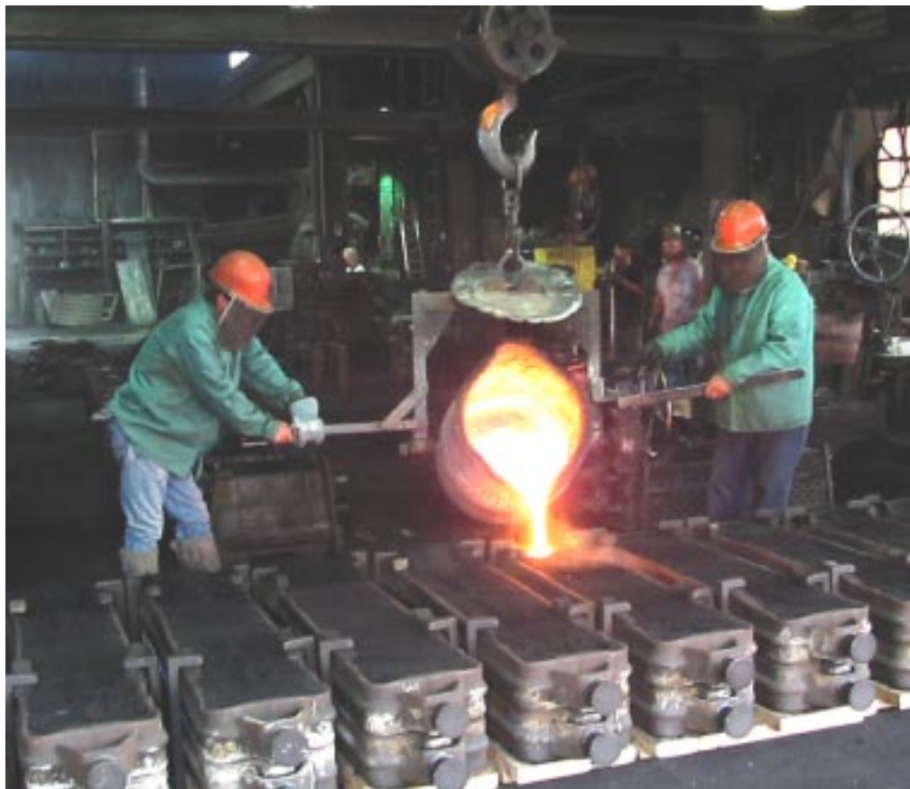
Photo 16. A pour directly from the large geared ladle. Depending on iron temperature and size of the molds, the iron remains hot enough to pour for about 20 minutes.
