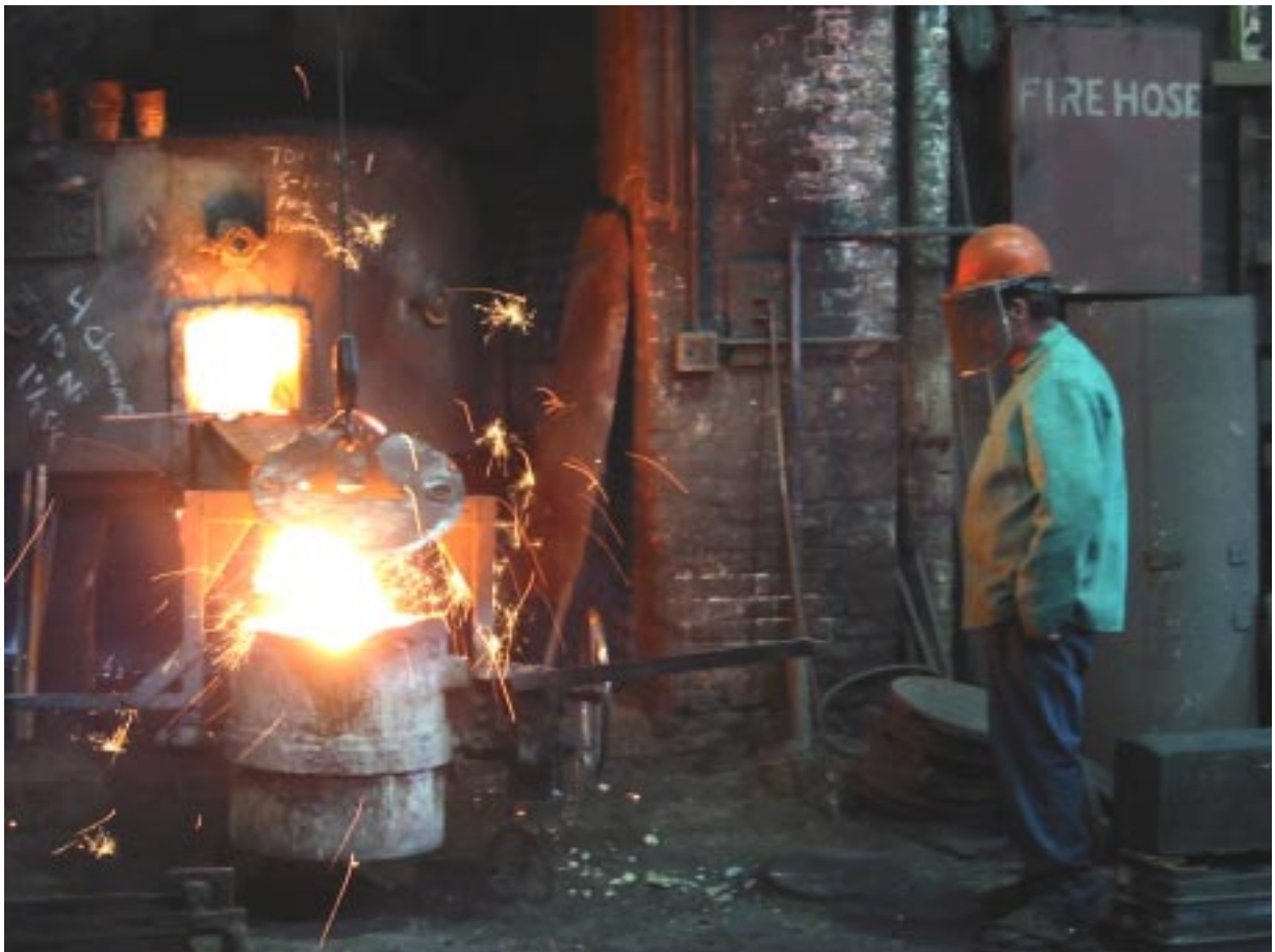
Photo 14. The cupola's tap hole open and iron flowing to the large geared ladle. This particular ladle has a capacity of 1,000 lbs.
