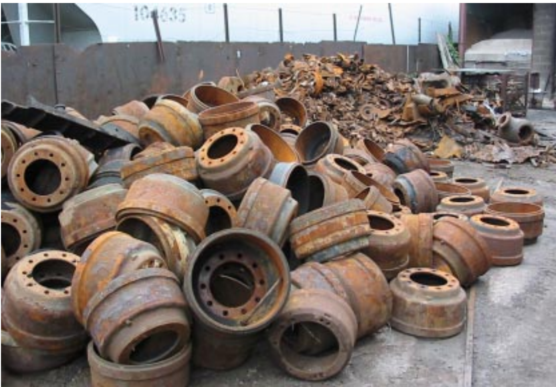
Photo 3. Scrap iron that comes from a local dealer. In the right background is storage for the daub used to repair the cupola's refractory lining.
