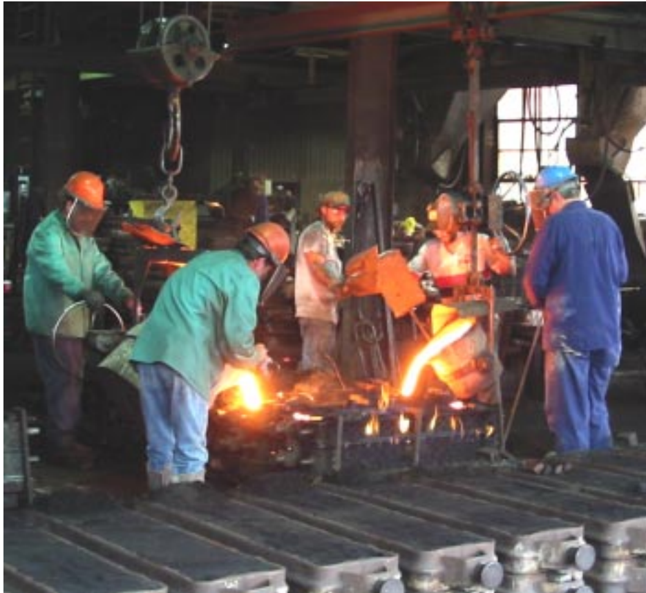
Photo 17. A "double pour" being made simultaneously from two ladles. Frank Doebler is at the far right.
