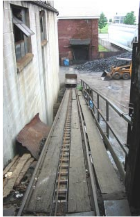
Photo 4. Views up and down the rails for cable car used to transport materials from ground level up to the cupola charging platform.
