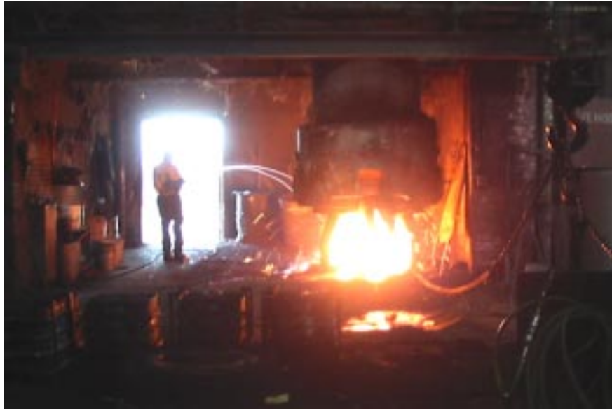
Photo 19. The scene a few seconds after the cupola had been dumped. Water is being sprayed onto the coke to quench the fire.
