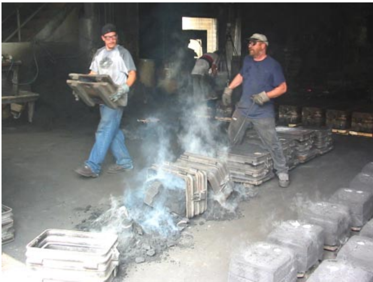
Photo 20. Shake-out beginning and bottom boards being gathered. The fumes are steam.
