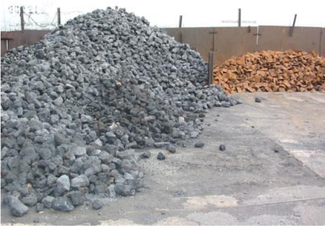
Photo 2. Piles of coke and pig iron. The coke is derived from bituminous coal mined in Kentucky, and the pig iron comes from Brazil.
