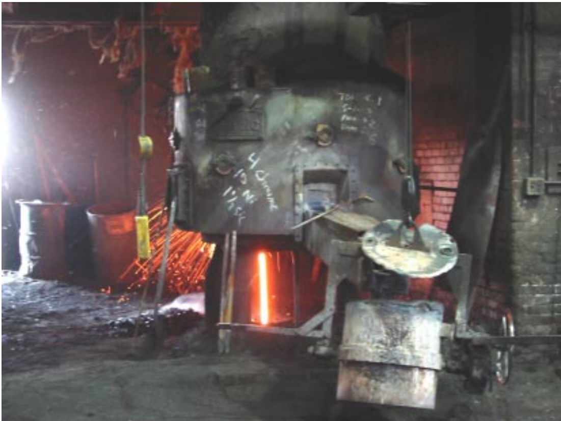
Photo 12. The cupola ready to be tapped and the ladle in position to receive the iron. On the opposite side of the cupola a stream of slag is pouring out the slag hole, and the sparkler effect indicates that iron also is reaching the height of the slag hole.
