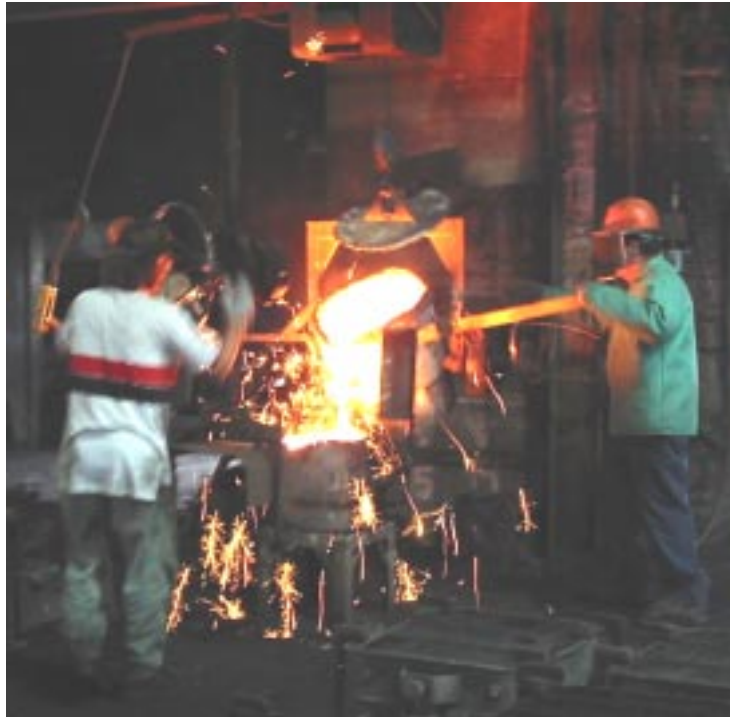
Photo 15. Iron being transferred to a smaller ladle for pouring.
