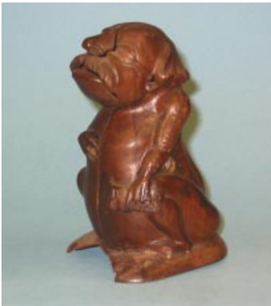
Photo 1. Wood master pattern for the "General Butler" bank, M-54.
