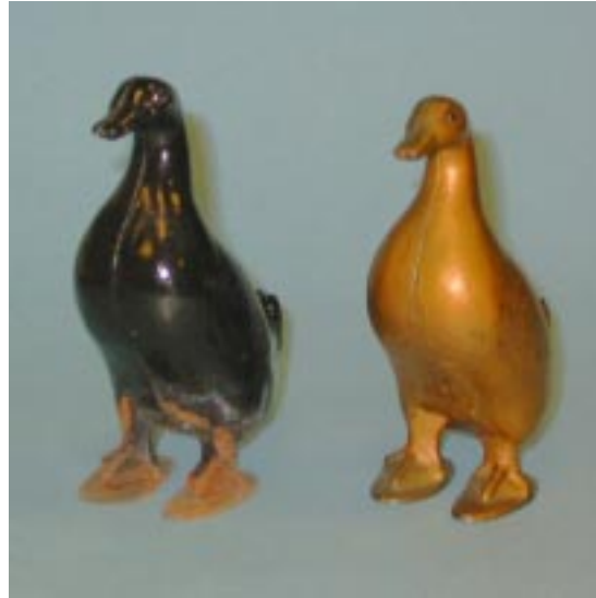
Photo 3. Wood master pattern (left) for the "Duck Bank", M-615, and example of cast iron bank.
