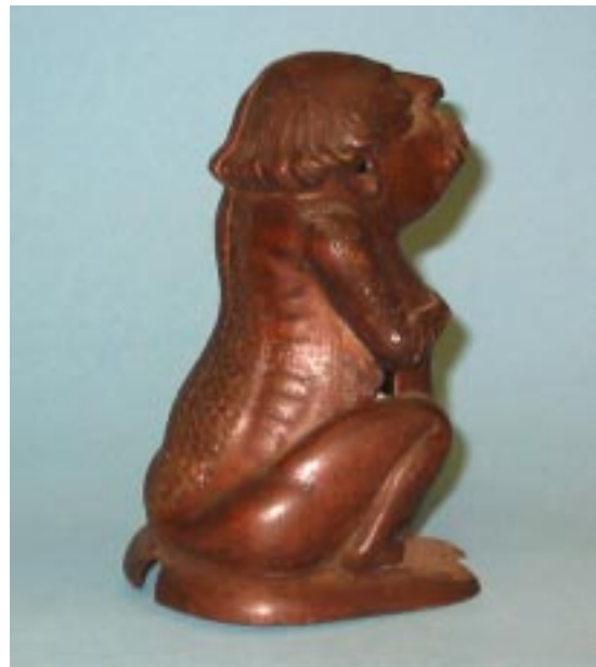
Photo 2. The gaps in the base front and back are where pieces of the pattern have broken off.
