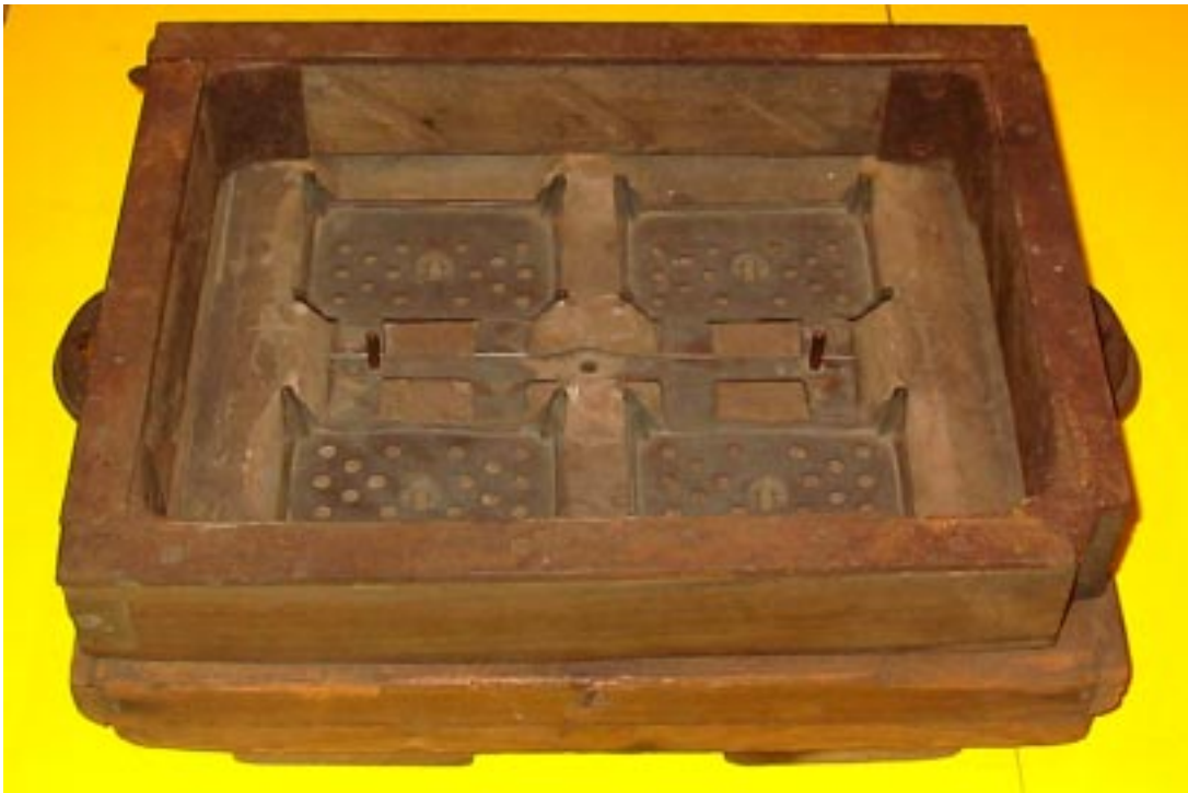
Photo 11. Match mold with the pattern tree in place.
