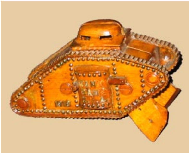
Photo 1. A.C. Williams' wood pattern for the "U.S. Tank Bank 1918," M-1437.
