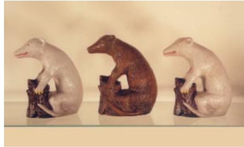
Photo 5. A.C. Williams' wood pattern and two trial iron castings for the proposed "Possum on Stump" bank.
