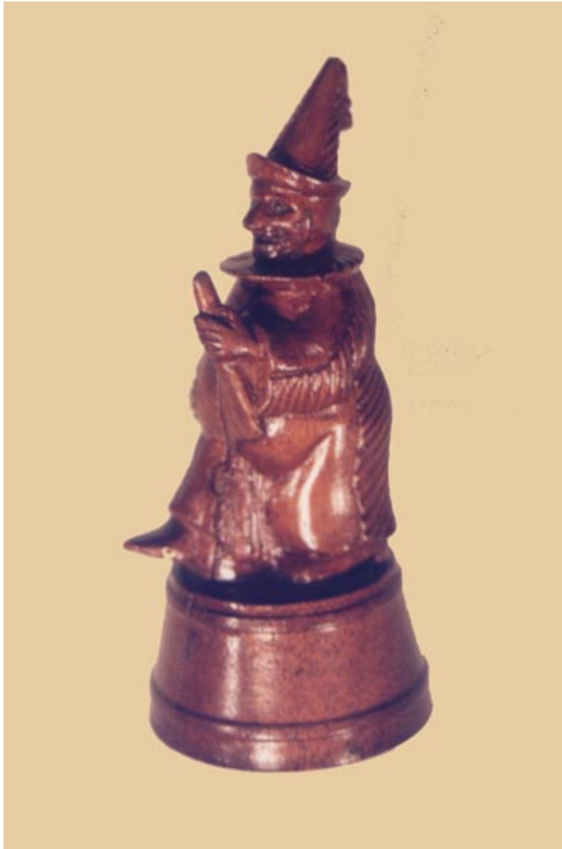
Photo 4. A.C. Williams' wood pattern for the proposed "Clown on Tub" bank.
